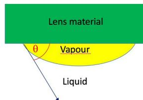
**Figure 2.** Diagrammatic representation of the captive bubble technique.  $\theta$  is the contact
