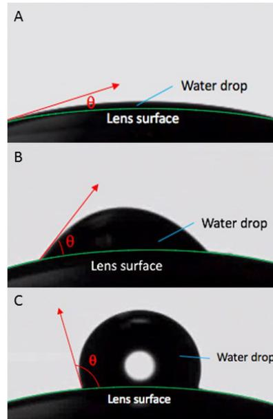
**Figure 1.** Examples of a contact lens with (A) a low contact angle ( $\theta$ ) and good wettability, (B) a higher contact angle and (C) a high contact angle with poor wettability obtained with the sessile drop technique.
